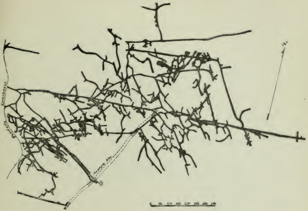
FIG. 17.—The drifts follow the lines of fissure as shown in the section in Fig. 16. The mine workings thus bring out clearly the fissure systems.
